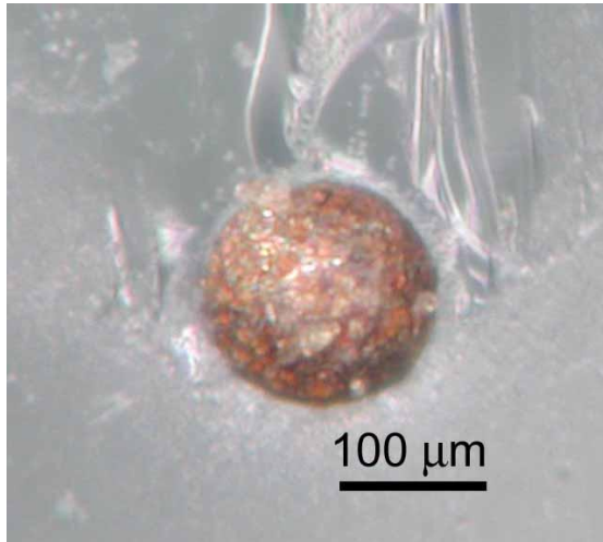
Nickel sulphide inclusions found on fracture surfaces of glass that failed by “spontaneous fracture”.
